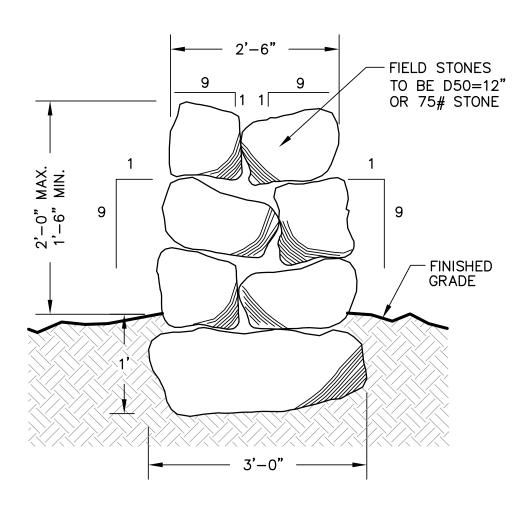
NOTE: STONES SHALL BE PLACED WITH A 1:9 CANT INWARD TOWARD THE CENTER OF THE WALL.
